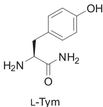
**Figure 3.** Chemical structure of L-Tym
