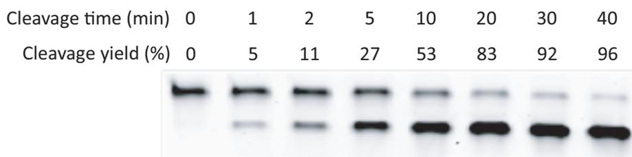
**Figure 5.** Monitoring the photocleavage of L-Tym biosensor using denaturing PAGE. (Reproduced from Tan et al, 2016, with permission from American Chemical Society).
